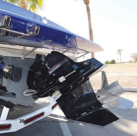
back, and we noticed that the aluminum hardware had been powdercoated rather than anodizing, which is sometimes a better choice, especially in the caustic Havasu water. The boat's rubrail is a plastic extrusion with a vinyl insert.
