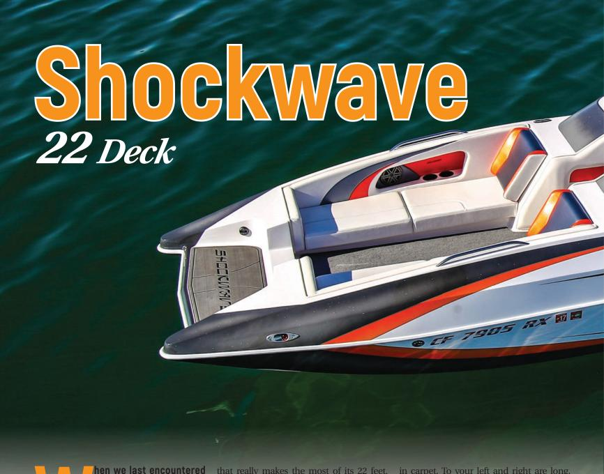
Shockwave's 22' Deck in 2016, it was in the form of a jetboat—power supplied by a Cadillac LS4 6.2 (550 hp) engine coupled to a Dominator jet. This year, company owner Bob Anderson brought us the same hull with a Mercury Racing 6.2—but with I/O power, the Bravo IV spinning a 22"-pitch prop. The drive might be different, but the fun has only improved. And if speed is your fun-measuring stick, guess what? We actually found another 2 mph.
